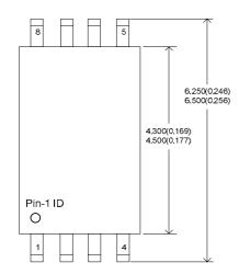
Dimensions are in milimeters(inches). Top line: (MIN) and Bottom line: (Max)
